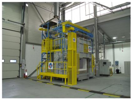
With the support of Catapult funding, the AFRC has become the owner of a new industrial gas furnace, a type widely used in industry. Within the forging industry, it can be used for preheating material and also for heat treatment purposes.
